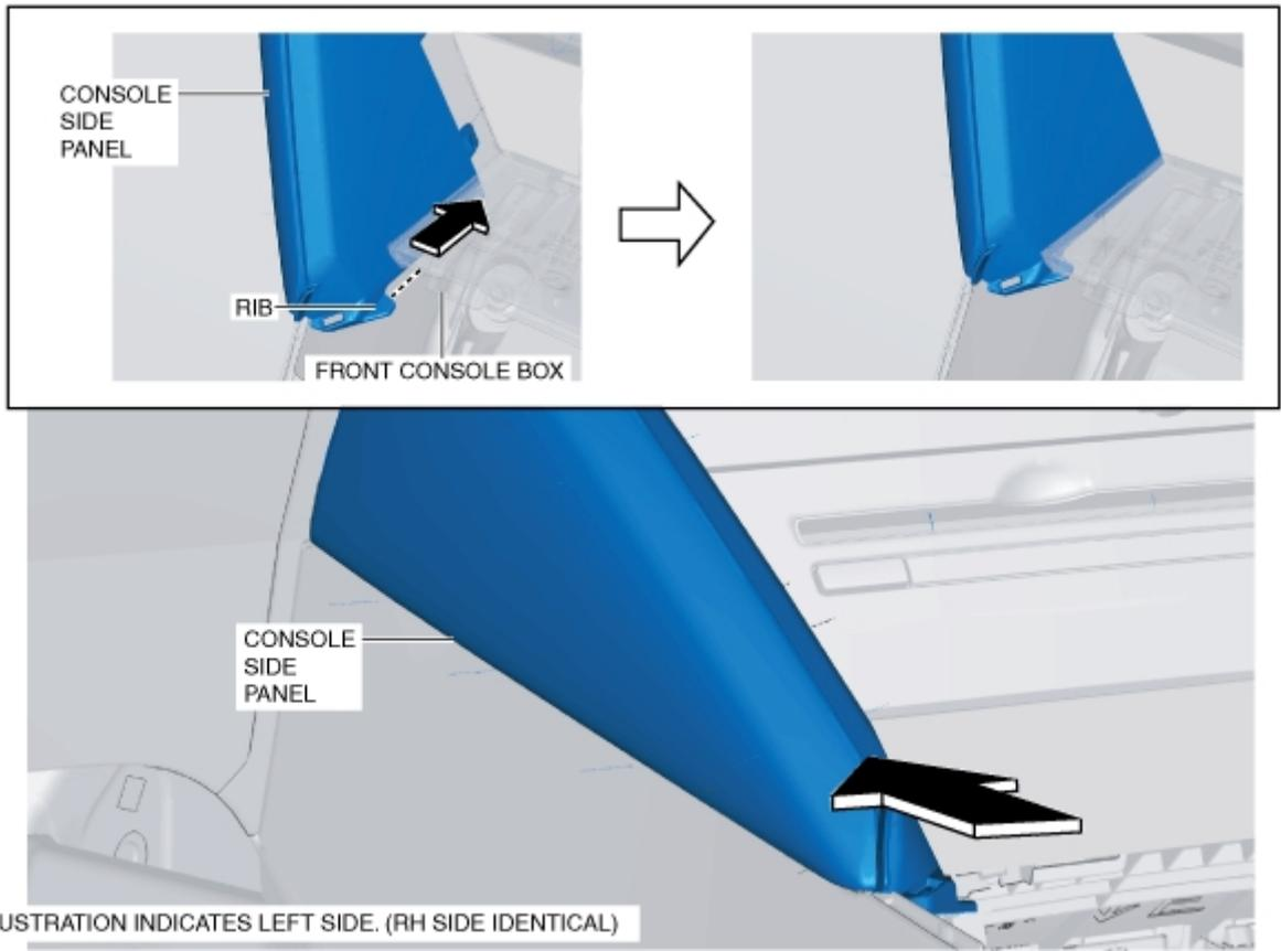
2. Align the installation positions of the clips and hooks, and install the console side panel in the direction of the arrow shown in the figure.
